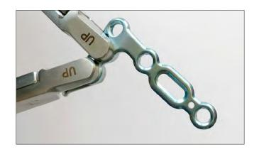
While bending, the plate must always be held at two adjacent holes to prevent contour deformation of the intermediate plate hole.
